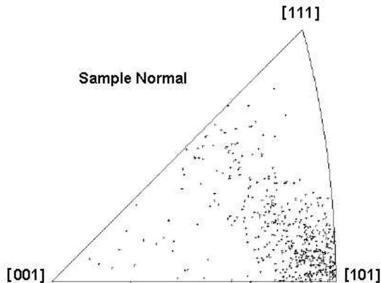
This example shows an Inverse Pole Figure containing a number of measurements for a cubic material.
