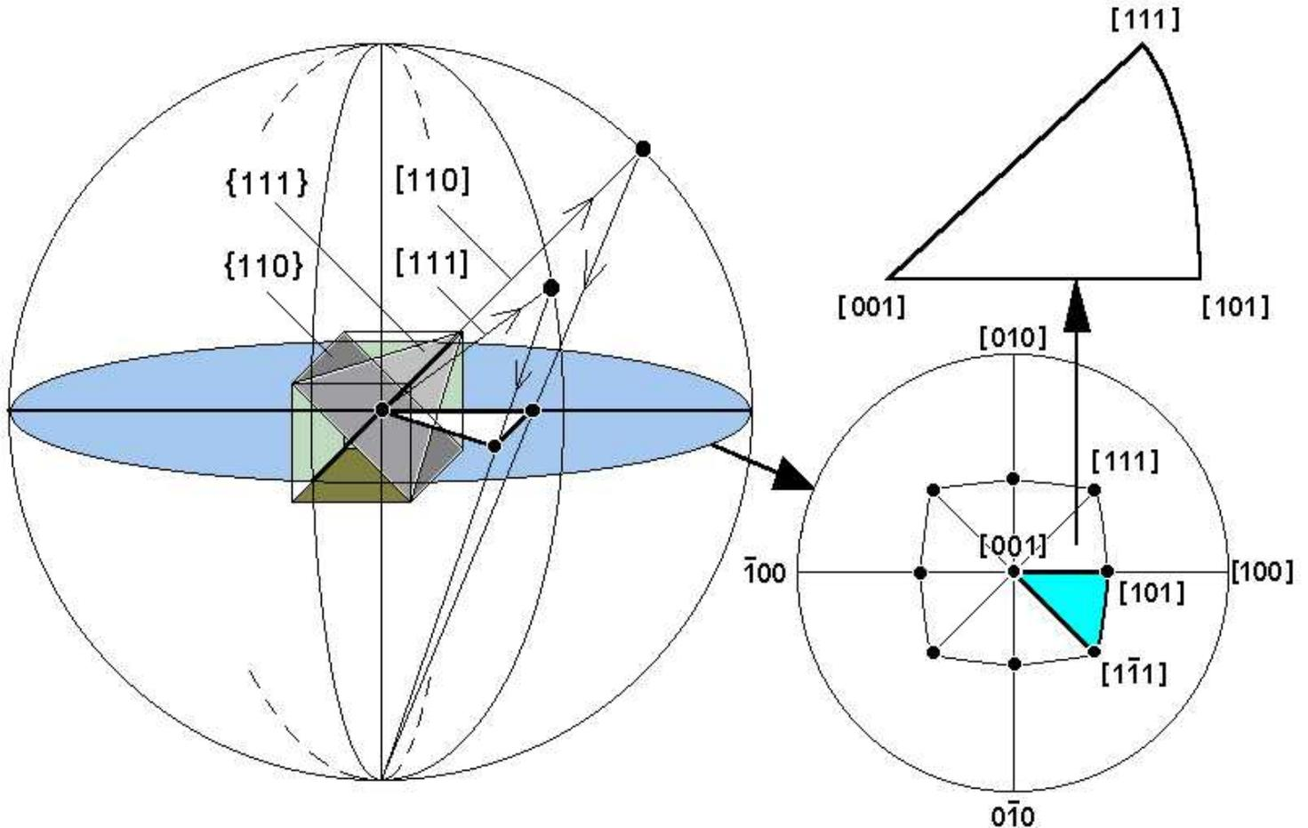
Because of the way the data is processed in an Inverse Pole Figure, each orientation is displayed as a single point, rather than a number of points as is the case with a Pole Figure. Inverse Pole Figures are commonly plotted for the Sample Normal Direction (ND), Rolling or Longitudinal Direction (RD/LD) and the Transverse Direction (TD).
