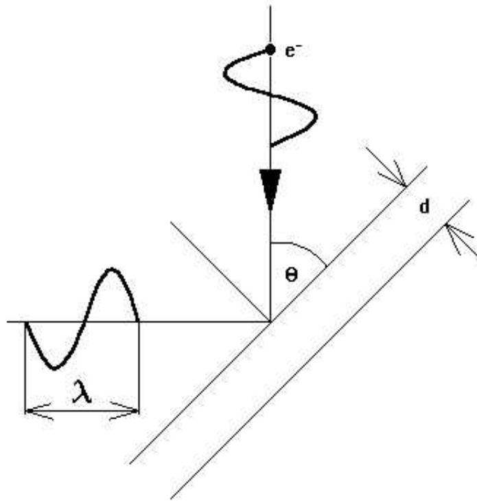
where  $n$  is the order of reflection,  $\lambda$  is the electron wavelength,  $d$  is the lattice spacing, and  $\theta$  is the Bragg angle, the angle of incidence of the electron.
