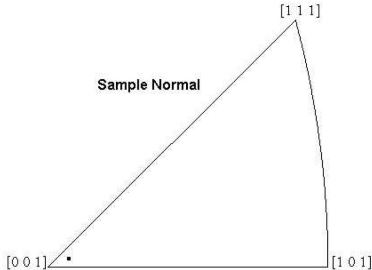
Considering the above Inverse Pole Figure plotted for the Sample Normal, the plot displays the orientation of the crystal directions with respect to the sample normal, i.e., that the observed orientation has the [001] direction close to the sample normal. For a cubic material, that implies that the (001) plane for that particular measurement lies close to parallel to the sample surface.
