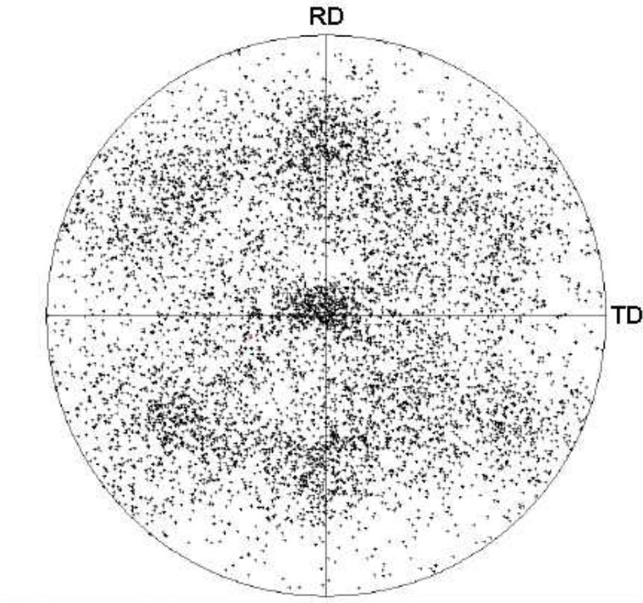
The Sample Normal Direction is represented by the center of the pole figure.
