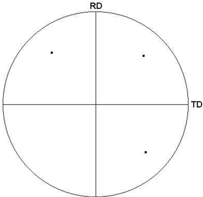
For each measurement on the sample, the different orientations alter the projected positions of the poles and hence different positions are plotted for the corresponding points in the projection plane. Thus a highly populated Pole Figure (one with many different measurements plotted) is useful for evaluating the orientation distribution:
