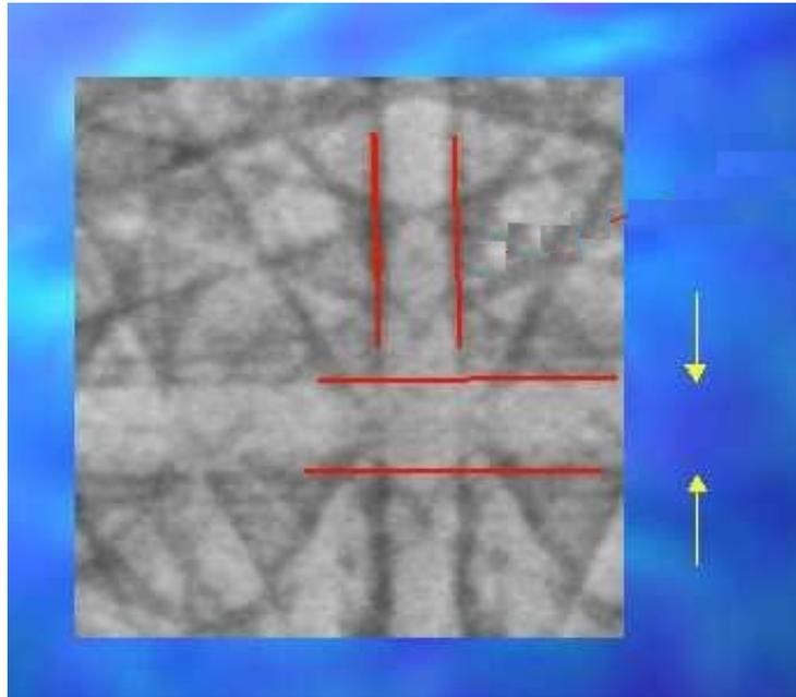
Bright 'Kikuchi' bands correspond to planes in the crystal lattice. The width of a band is dependent upon the electron wavelength and lattice plane spacing.
