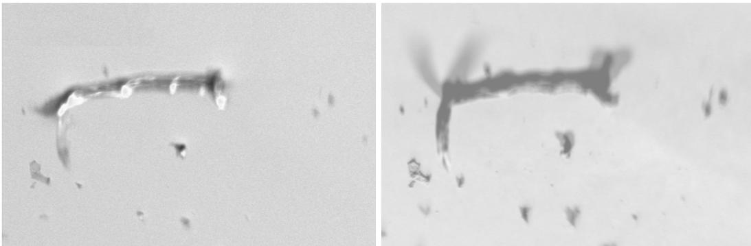
The electron image on the left comes directly from the microscope. The image on the right is from two detector diodes, but their slightly different positions create two shadows in a "V" shape in the combined image. This can give a false impression of the real artefacts.
