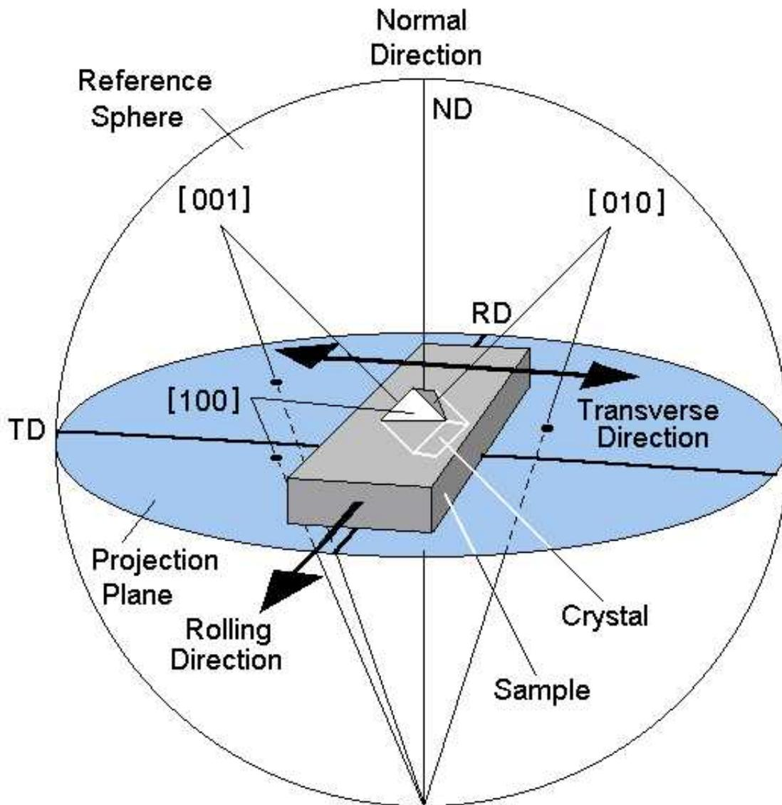
Thus for a 100 Pole Figure, each measurement will result in multiple points in the equatorial or projection plane:
