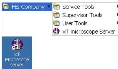
The **xT microscope Server** application starts and stops the software service controlling basic microscope functions and also the user interface (UI) software **xT microscope Control**.
