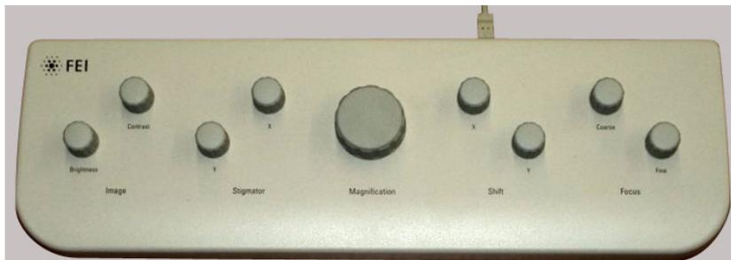
The MUI offers additional flexibility for controlling magnification, beam shift, focus, astigmatism, contrast and brightness.
