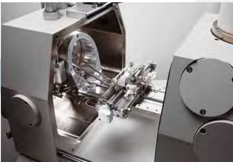
SEM chamber and stage.
