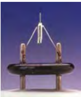
A FIB's liquid metal ion source (LMIS).
