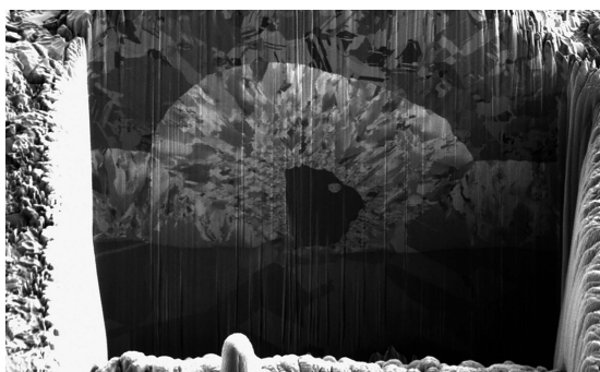
Cross section of defect buried below the surface in a ceramic sample.
