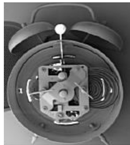
Wide-field SE imaging in TESCAN Mira3 SEM demonstrating the ability to examine large objects.
